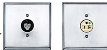
HBL24300RKS Single retrofit accepts hospital only Hubbellock single receptacles (Hubbell HBL23000HG) or 20A single straight blade hospital grade receptacles (Hubbell HBL8310, HBL8310I, IG8310, etc.). Order receptacles separately.
